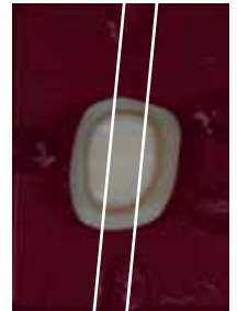
Placement of cuts parallel to the milling direction
