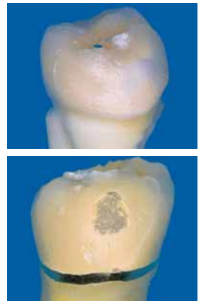
Typical failure pattern of veneering ceramic in one all-ceramic and one metal-ceramic restoration after fracture load testing.
